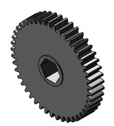
Diametral pitch: 20 Pressure angle: 14.5 Number of teeth: 45 Pitch diameter: 2.25 inch
